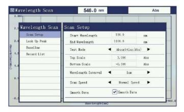
To test sample solution absorbance peak, can scan the sample characteristic curve of any wavelength range between 190 and 1100nm. You can look up the peak value on the standalone device.
