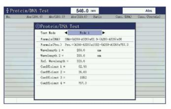
There are two test modes and formulas based on absorbance ratio 260nm/280nm or 230nm with substracted absorbance at 320nm.
