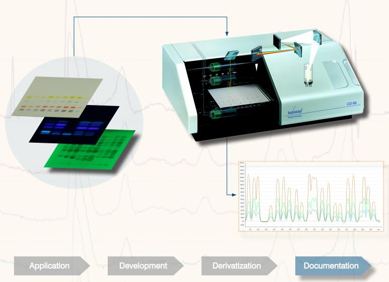
For quantitative determination of samples, the HPTLC-Densitometer CD60 converts the spots/bands of the single substances into a chromatogram curve. It measures the absorbance or fluorescence of separated compounds in transmission or reflection mode. The HPTLC-Densitometer CD60 is controlled by ProQuant software which also enables quantitative evaluation of the generated data.
