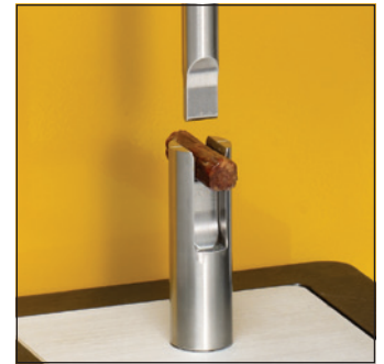
TA-VBJ F Volodkevich Bite Jaws for testing bite force of meat products using shear cutting-test. Fixture Base Table required.
