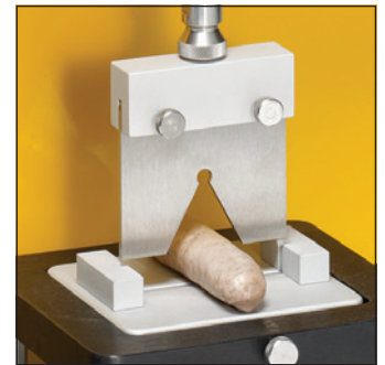
TA-SBA-WB-1 F 1mm Shear Blades for cutting-shear test: meat, fish, sausage, etc. TA-SBA-WB-3 option for 3mm blades. Fixture Base Table required.
