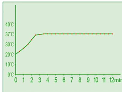
Quickly heating up and thermostable technique to ensure reaction solution reach  $37\pm 0.5^{\circ}\text{C}$  within 160s and stable at  $37\pm 0.2^{\circ}\text{C}$  more than 1200s.
