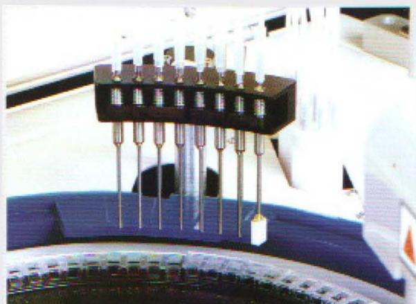
An 8-channel washing station ensures complete washing for cuvettes.
