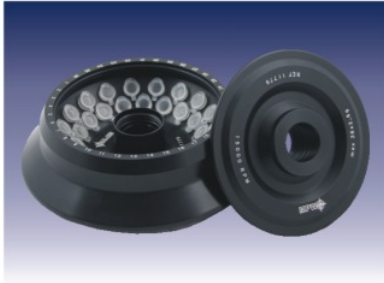
Angle rotor 36x2,2ml, with filter, with HS*, No 11779, max. speed 15 000 rpm, RCF 22 136xg, Max. radius R= 8,8 cm, angle 45°
