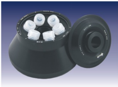
Angle rotor 6x50ml Nalgene, with HS*, No 11773, max. speed 14 500 rpm, RCF 21 625xg, Max. radius R= 9,2 cm, angle 30°
