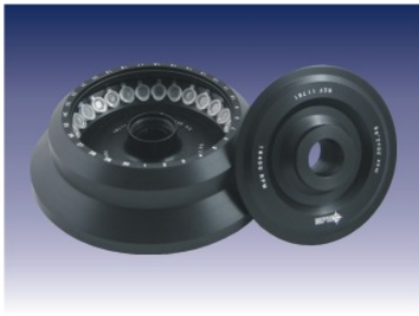
Angle rotor 30x2,2/1,5ml, with HS*, No 11761, max. speed 16 400 rpm, RCF 29 168xg, Max. radius R= 9,7 cm, angle 45°
