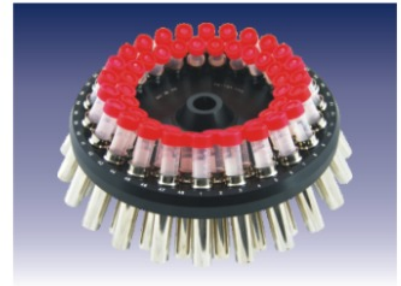
Angle rotor 48x15ml Falcon, No 11785, max. speed 4 700 rpm, RCF 4 025xg, Max. radius R= 16,3 cm, angle 30°
