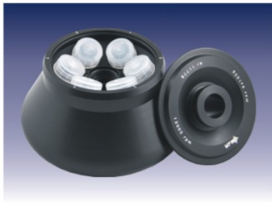
Angle rotor 6x94/85ml Nalgene, with HS*, No 11778, max. speed 12 000 rpm, RCF 17 710xg, Max. radius R= 11 cm, angle 30°
