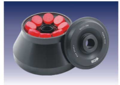
Angle rotor 8x50ml Falcon, with HS*, No 11776, max. speed 14 000 rpm, RCF 23 666xg, Max. radius R= 10,8 cm, angle 30°
