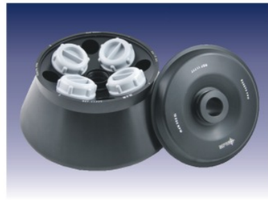
Angle rotor 4x250ml Nalgene, with HS*, No 11777, max. speed 10 000 rpm, RCF 14 086xg, Max. radius R= 12,6 cm, angle 25°
