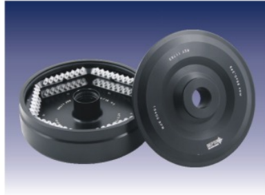
Angle rotor 12x8x0,2ml PCR, with HS*, No 11765, max. speed 16 400 rpm, RCF 28 566xg, Max. radius R= 9,5 cm, angle 45°
