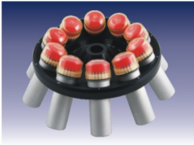
Angle rotor 12x50ml Falcon, No 11780, max. speed 4 500 rpm, RCF 3 328xg, Max. radius R= 14,7 cm, angle 30°
