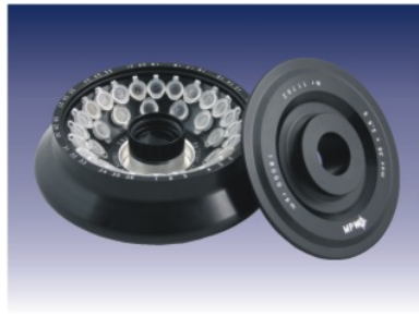
Angle rotor 36x2,2/1,5ml, with HS*, No 11762, max. speed 18 000 rpm, RCF 30 065xg, Max. radius R= 8,3 cm, angle 45°
