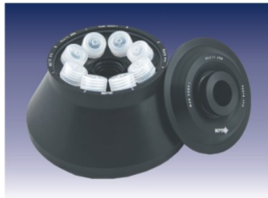
Angle rotor 8x50ml Nalgene, with HS*, No 11775, max. speed 14 000 rpm, RCF 21 255xg, Max. radius R= 9,7 cm, angle 30°
