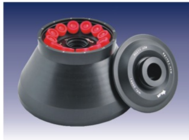
Angle rotor 12x15ml Falcon, with HS*, No 11770, max. speed 14 000 rpm, RCF 23 227xg, Max. radius R= 10,6 cm, angle 30°
