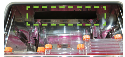
Top side of Chamber Airflow Duct and Sensors
