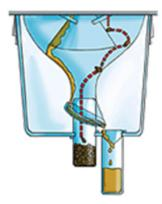
Urine flows along the inside surface of the **collection funnel** and is directed by the urine ring directly into the urine collection tube.
